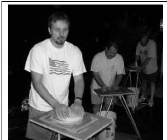
Mike Lindner fine-grinding an element of his anastigmat corrector. STAR President Greg Cantrell and Steve Fedor in background
